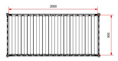
L: 2112mm H: 855mm D: 978mm INNERSIZE 2000x900mm
