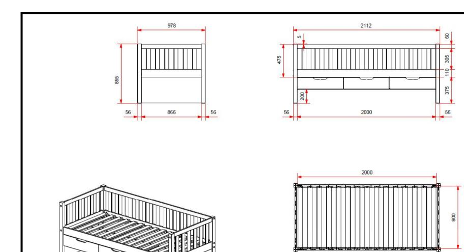
L: 2112mm H: 855mm D: 978mm INNERSIZE 2000x900mm
